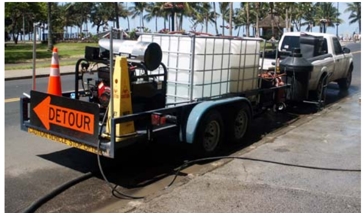
WBIDA's new water recovery and recycling system
